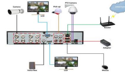
**Figure 2-1 Device Connection**
